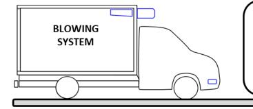
At the warehouse the refrigeration unit will operate connected to the mains. During the delivery round, it will be driven by the vehicle's energy, the engine of which must be in service so that the group itself can operate.
