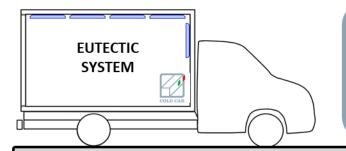
The refrigeration unit is electric only and will only work during the night, connected to the mains. It will lower the temperature of the eutectic liquid to -38°C/-36,4°F and the body's internal temperature to -33°C/-27,4°F
