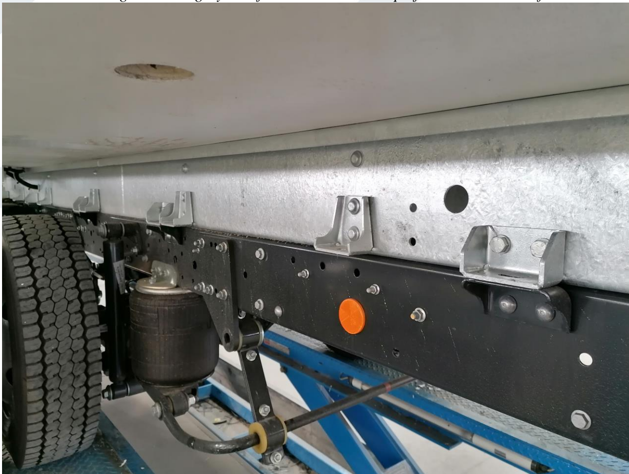
Cold Car galvanized grey Sub-frame installed on top of the chassis black frame
