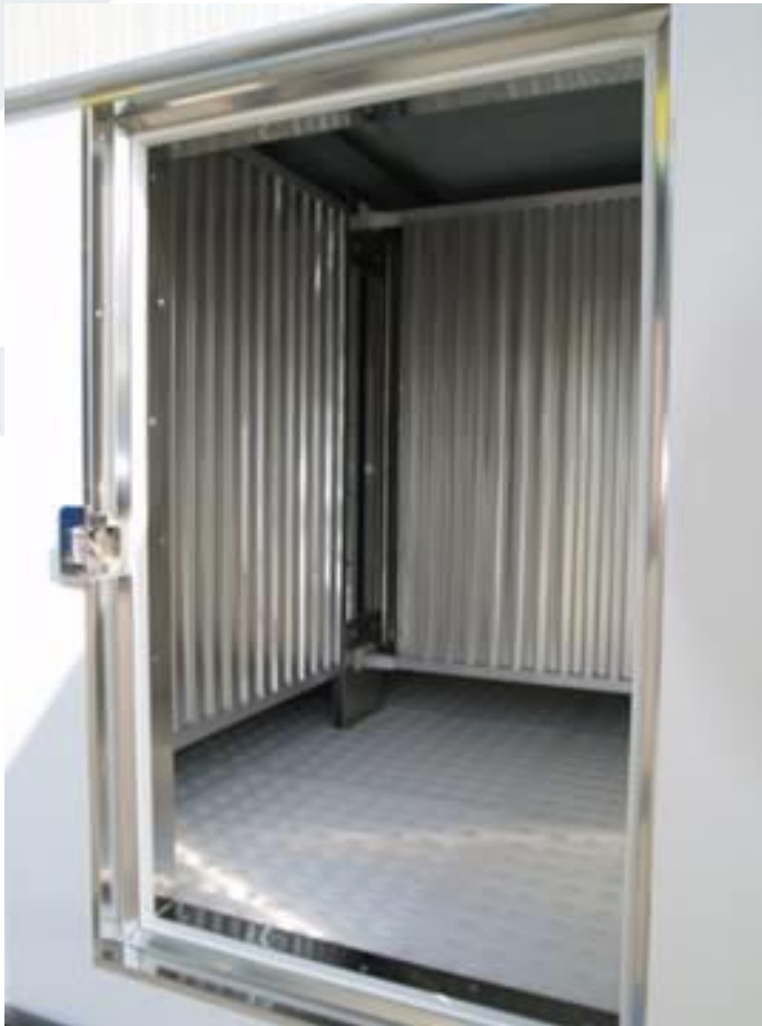
Side door view with Aluminum dividers and plastic grating on the floor
