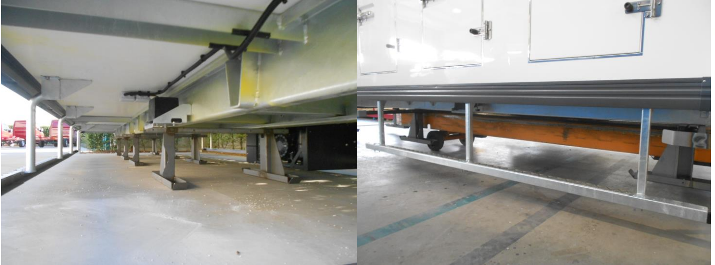
Galvanized sub-frame and side footboards under the floor
